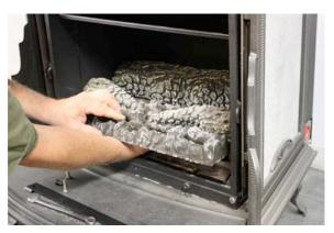
6. Lift the burner out of the firebox. Lift the front edge first then pull it up and out of the firebox. Natural gas stoves will have a narrow air shield attached to the burner. (see picture on the next page)
